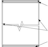
Hanging kit (hangers) to be fitted flush with the top of the panel.
