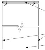
Hangers to be fitted flush with the top ~ and sides of the panel. If a smaller or less rigid 'D' end panel is required, the end hangers can be cut down using a sharp pair of scissors. End sections – minimum length of 70mm each.
